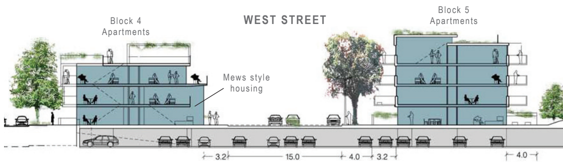
Cross section through West street -Alternative with Mews style housing to block 4
